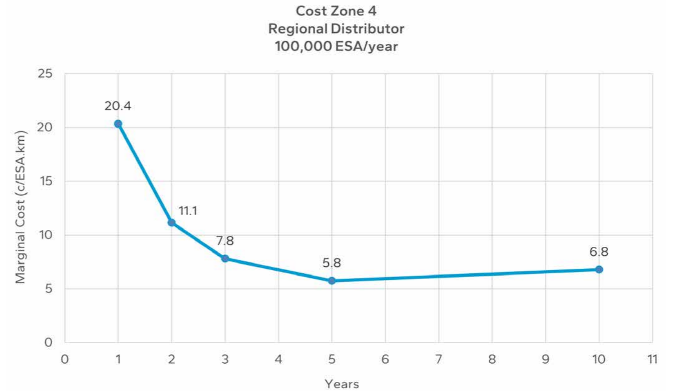
Figure B 15.3: Marginal cost chart for cost zone 4 regional distributor roads with 100,000 ESA/year loading
