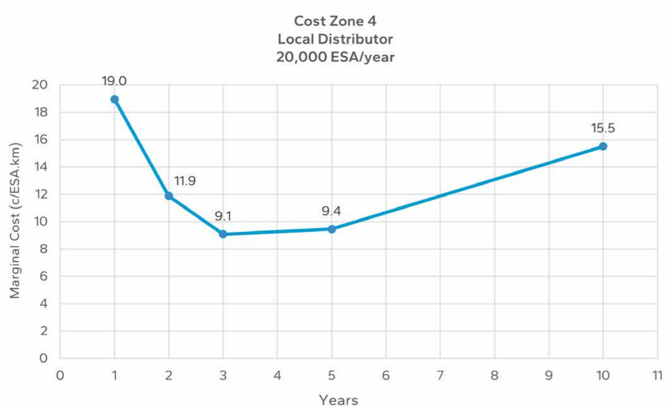
Figure B 14.1: Marginal cost chart for cost zone 4 local distributor roads with 20,000 ESA/year loading
