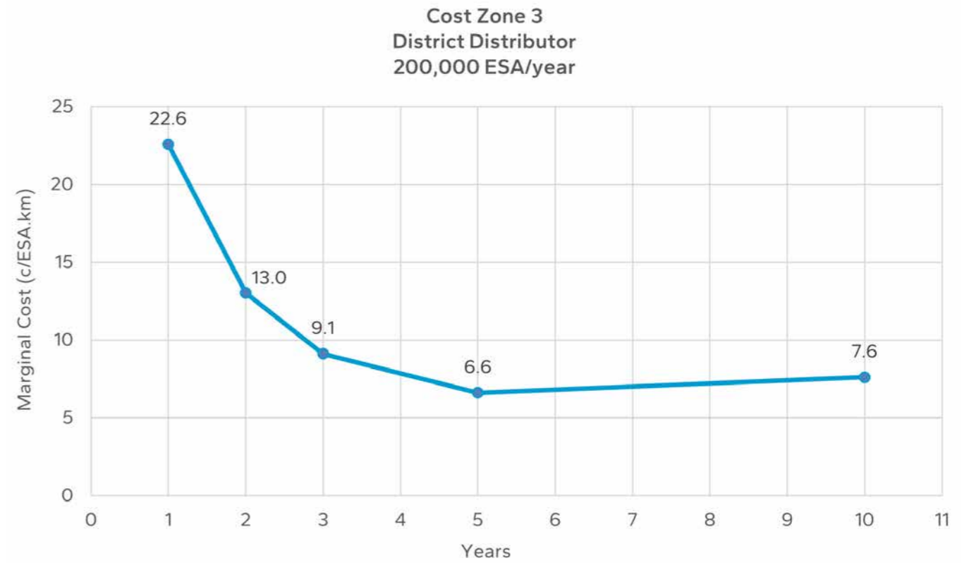
Figure B 12.4: Marginal cost chart for cost zone 3 district distributor roads with 200,000 ESA/year loading
