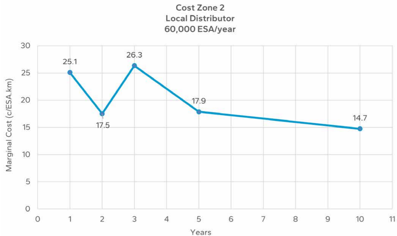
Figure B 6.2: Marginal cost chart for cost zone 2 local distributor roads with 60,000 ESA/year loading
