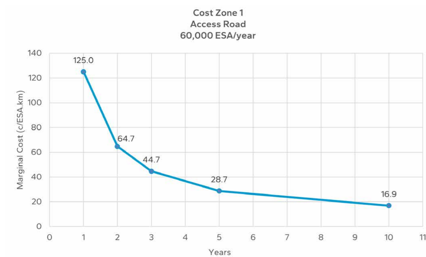
Figure B 1.2: Marginal cost chart for cost zone 1 access roads with 60,000 ESA/year loading
