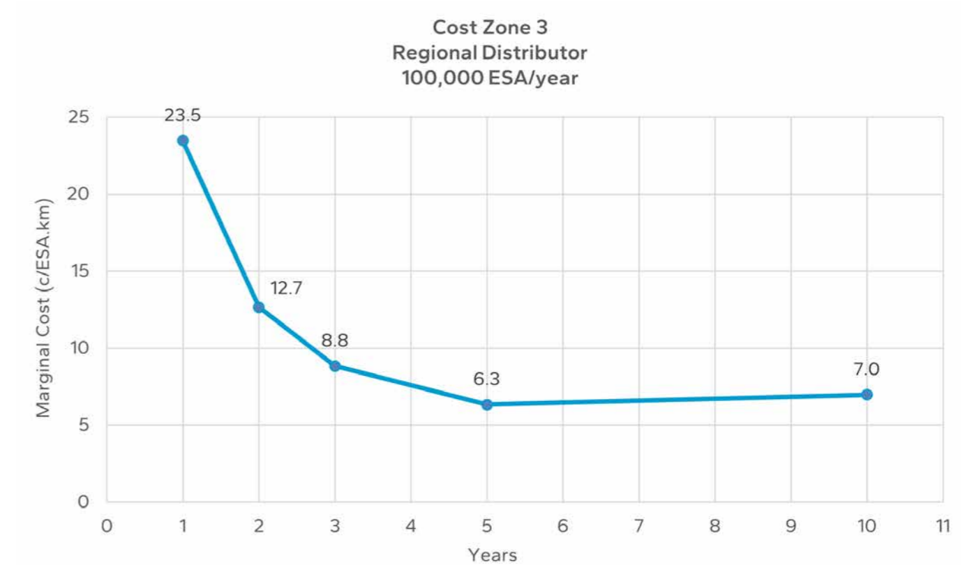
Figure B 11.3: Marginal cost chart for cost zone 3 regional distributor roads with 100,000 ESA/year loading
