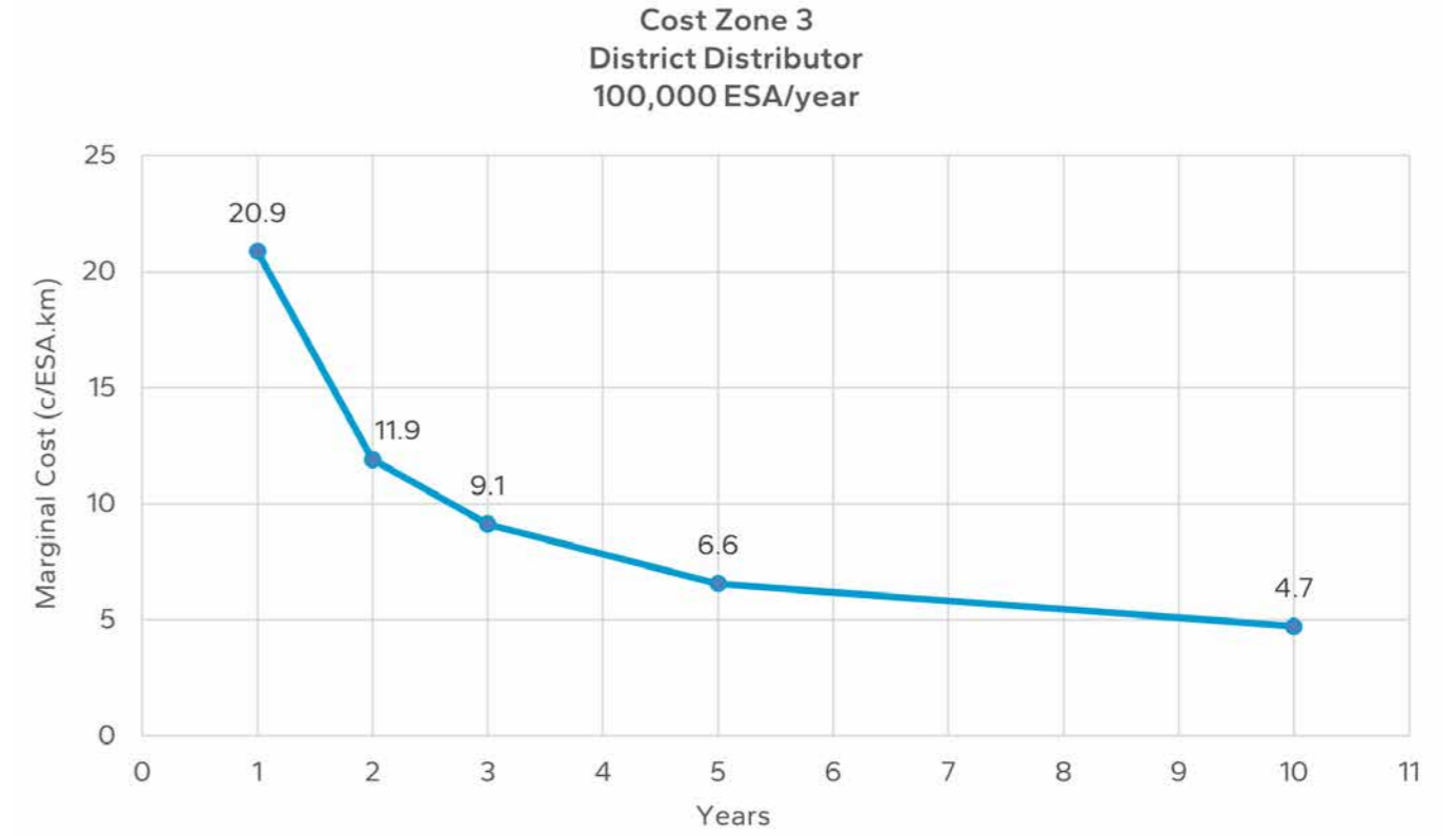
Figure B 12.3: Marginal cost chart for cost zone 3 district distributor roads with 100,000 ESA/year loading
