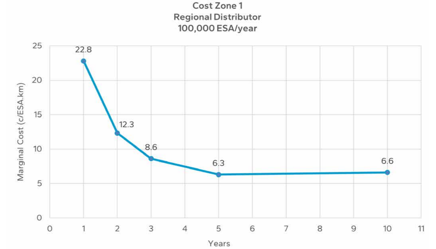
Figure B 3.3: Marginal cost chart for cost zone 1 regional distributor roads with 100,000 ESA/year loading
