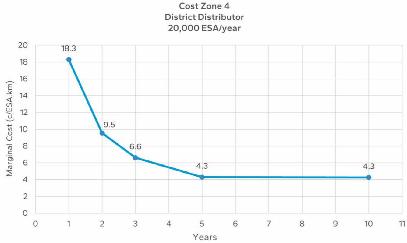
Figure B 16.1: Marginal cost chart for cost zone 4 district distributor roads with 20,000 ESA/year loading
