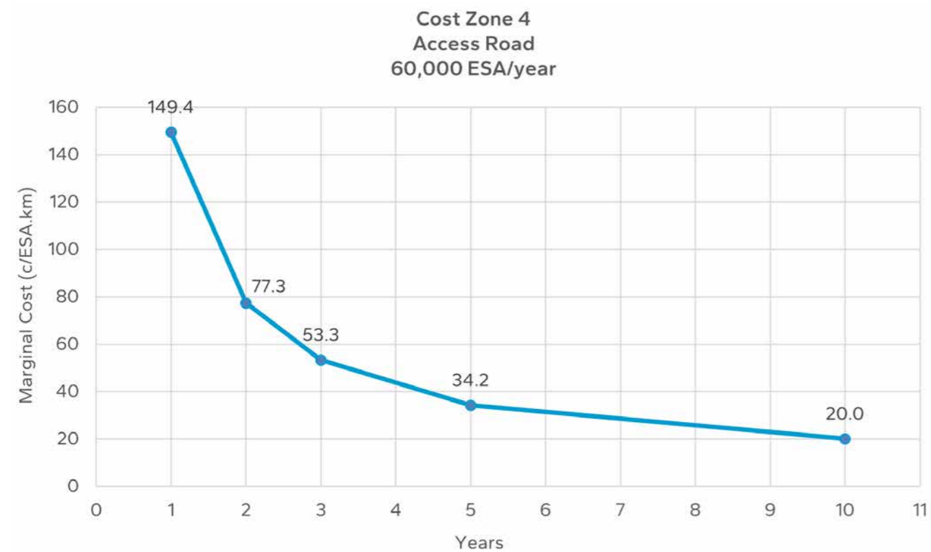
Figure B 13.2: Marginal cost chart for cost zone 4 access roads with 60,000 ESA/year loading
