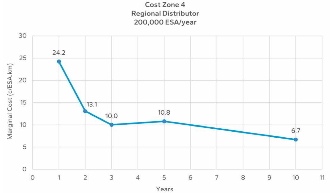
Figure B 15.4: Marginal cost chart for cost zone 4 regional distributor roads with 200,000 ESA/year loading
