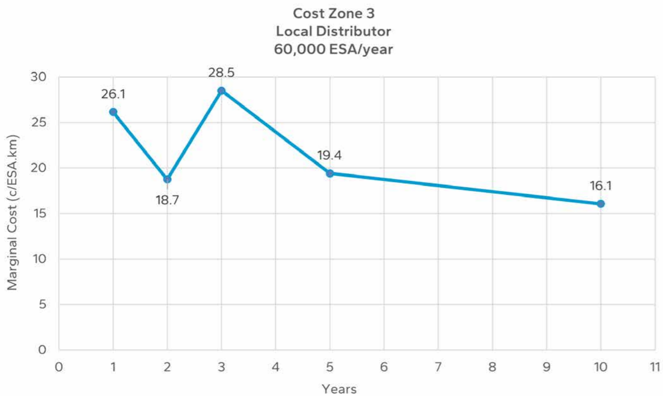
Figure B 10.2: Marginal cost chart for cost zone 3 local distributor roads with 60,000 ESA/year loading
