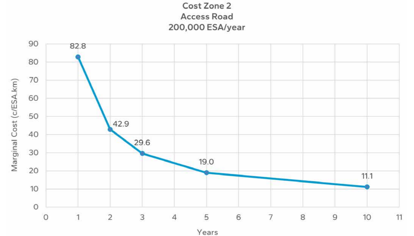
Figure B 5.4: Marginal cost chart for cost zone 2 access roads with 200,000 ESA/year loading
