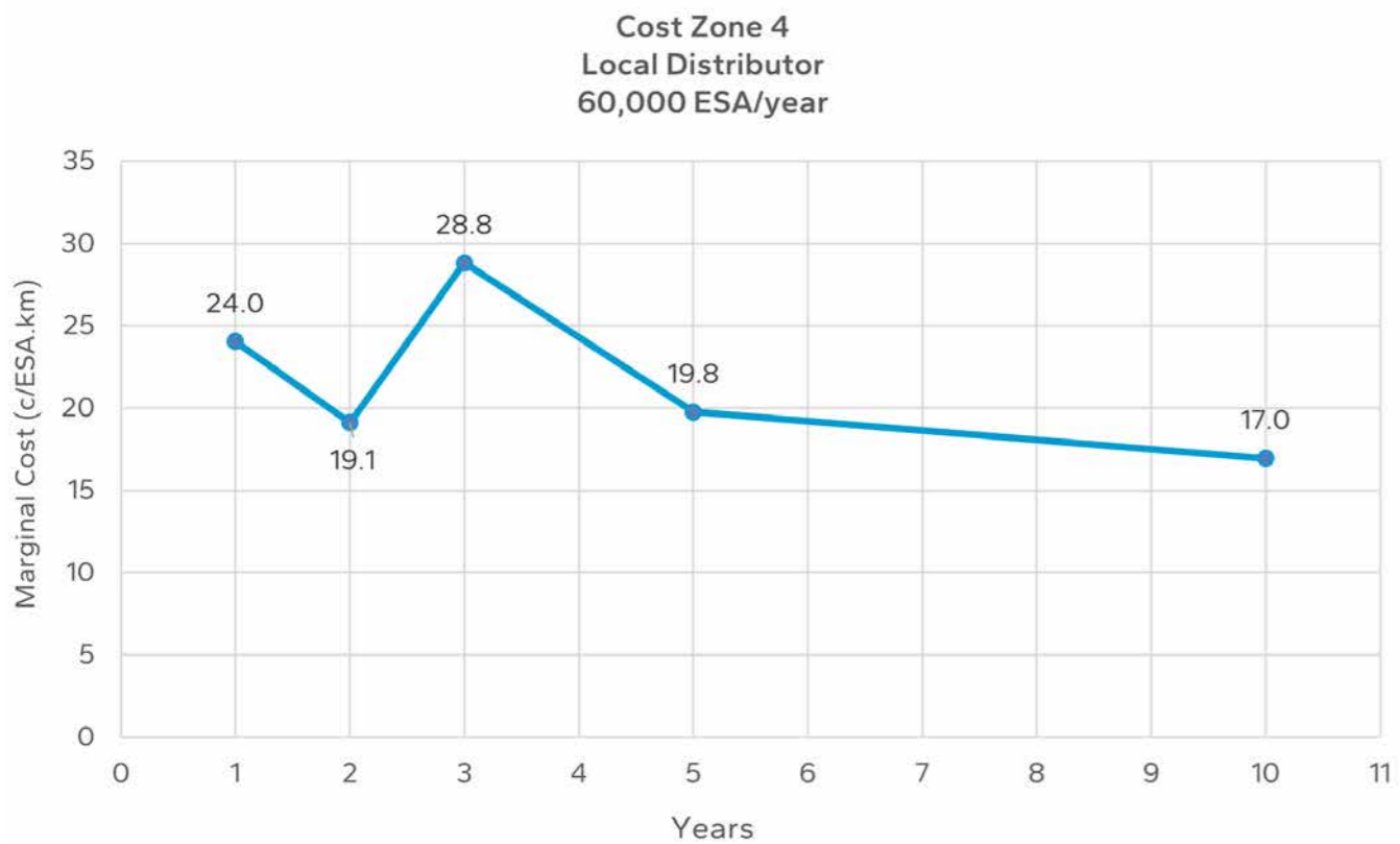
Figure B 14.2: Marginal cost chart for cost zone 4 local distributor roads with 60,000 ESA/year loading
