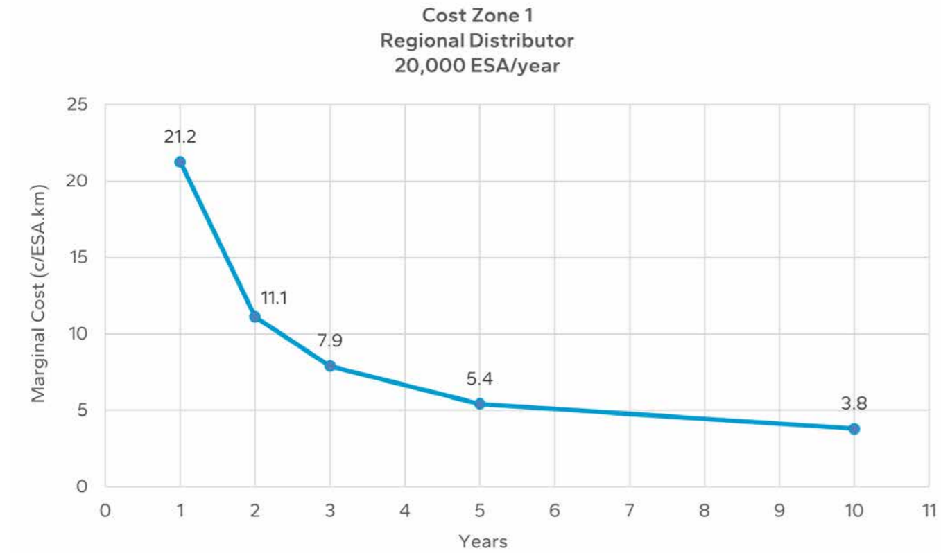
Figure B 3.1: Marginal cost chart for cost zone 1 regional distributor roads with 20,000 ESA/year loading
