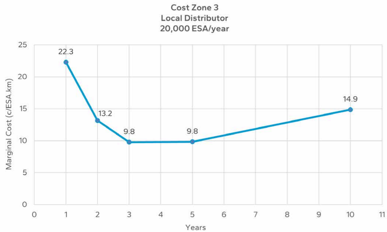
Figure B 10.1: Marginal cost chart for cost zone 3 local distributor roads with 20,000 ESA/year loading
