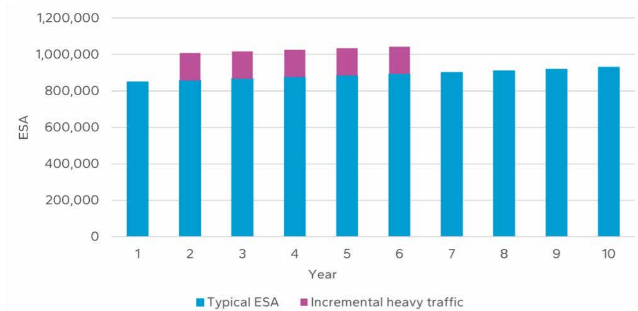
Figure C.1: Traffic load versus time showing a typical additional load for a set duration
