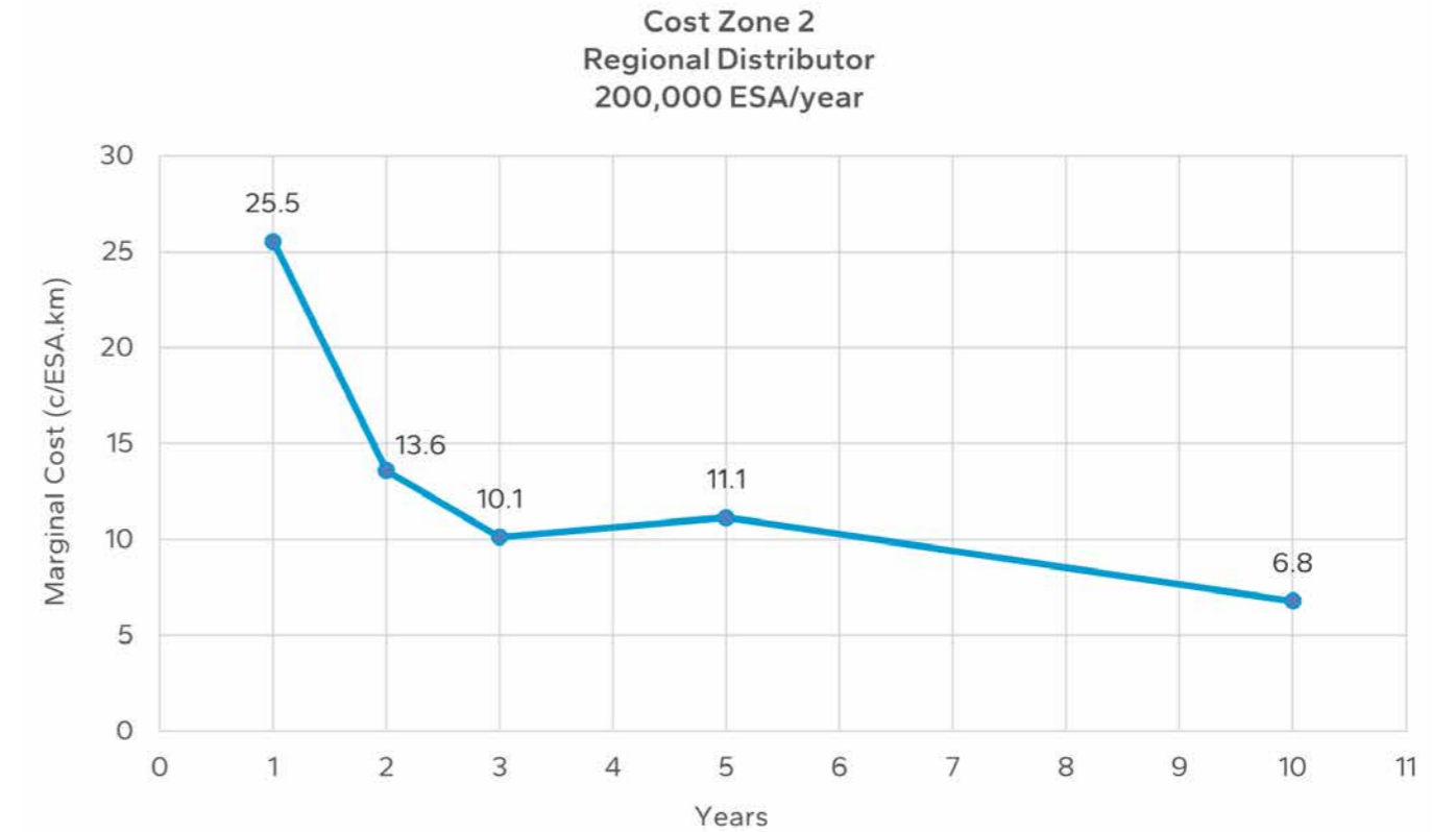
Figure B 74: Marginal cost chart for cost zone 2 regional distributor roads with 200,000 ESA/year loading
