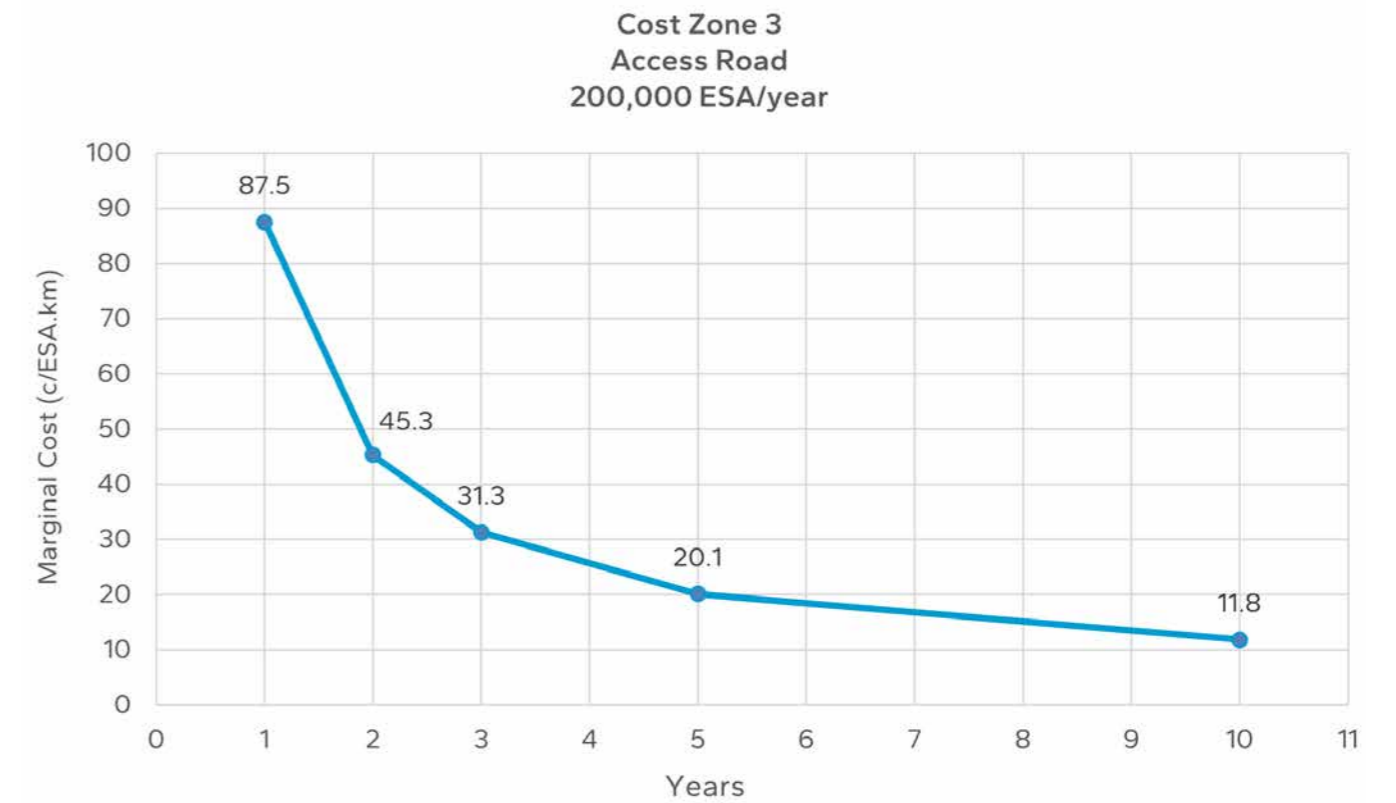
Figure B 9.4: Marginal cost chart for cost zone 3 access roads with 200,000 ESA/year loading
