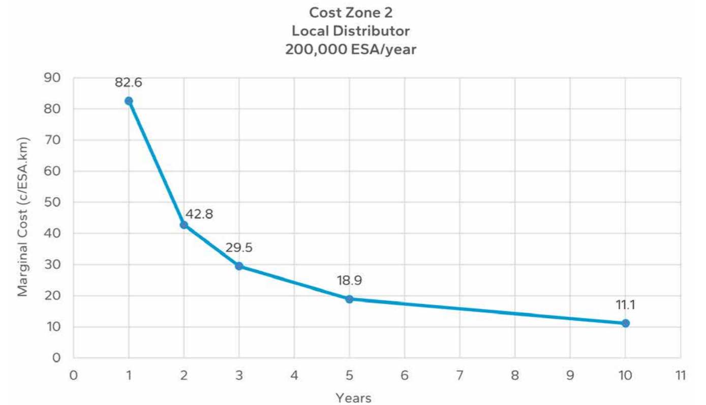
Figure B 6.4: Marginal cost chart for cost zone 2 local distributor roads with 200,000 ESA/year loading
