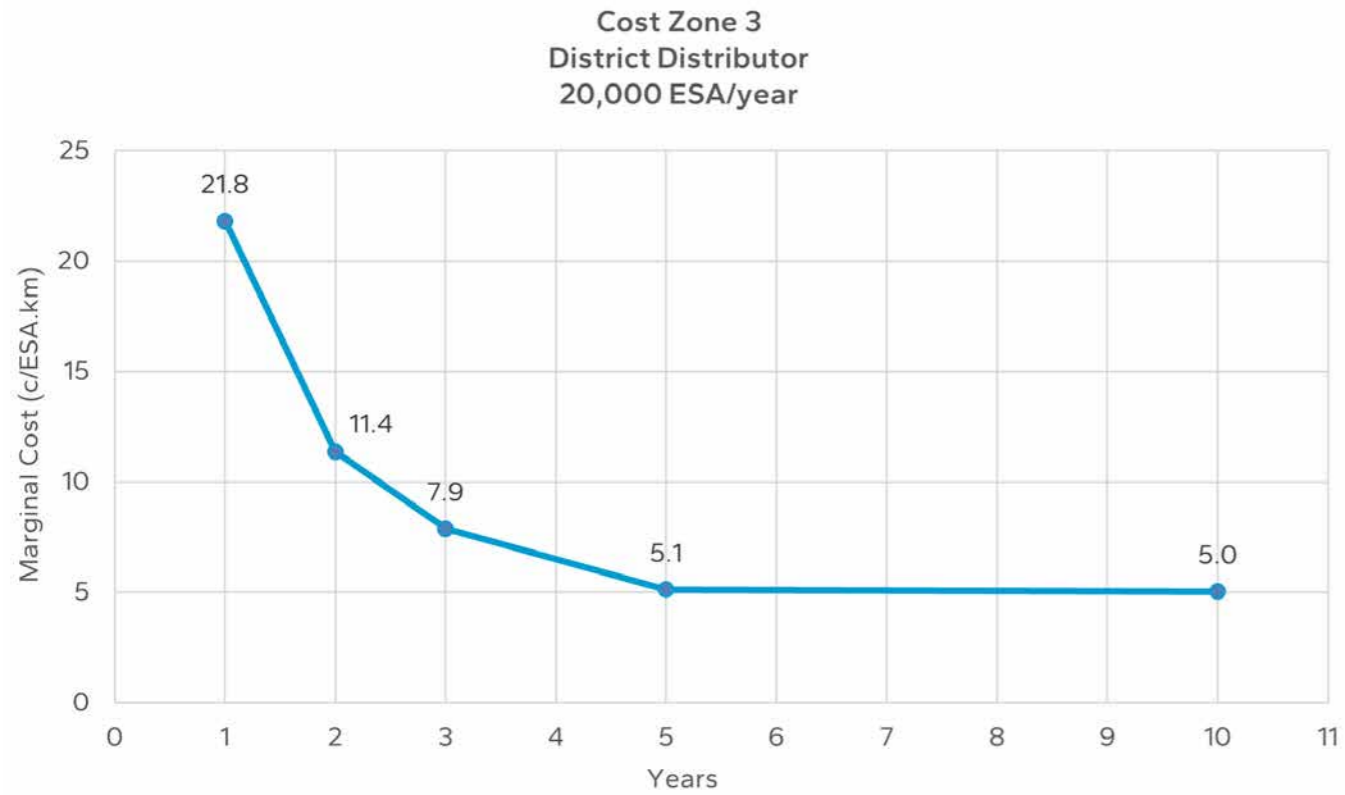
Figure B 12.1: Marginal cost chart for cost zone 3 district distributor roads with 20,000 ESA/year loading
