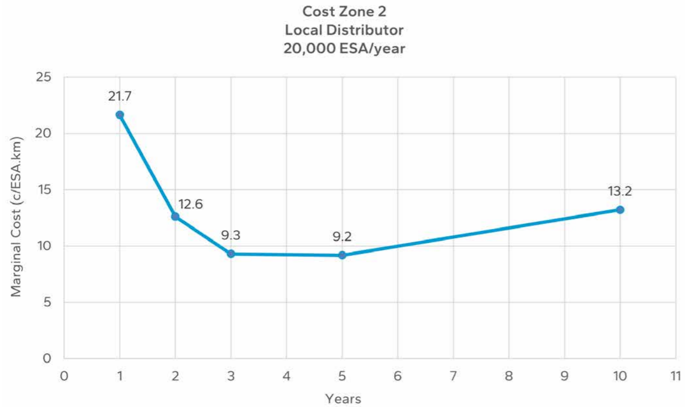
Figure B 6.1: Marginal cost chart for cost zone 2 local distributor roads with 20,000 ESA/year loading
