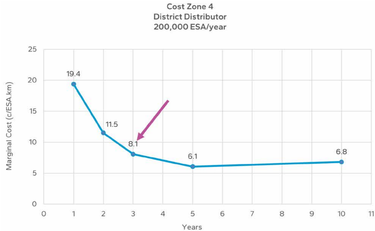
Figure 6: Marginal cost chart of a district distributor in cost zone 4 with an additional 200,000 ESA/year
