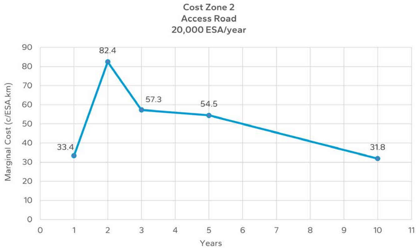
Figure B 5.1: Marginal cost chart for cost zone 2 access roads with 20,000 ESA/year loading
