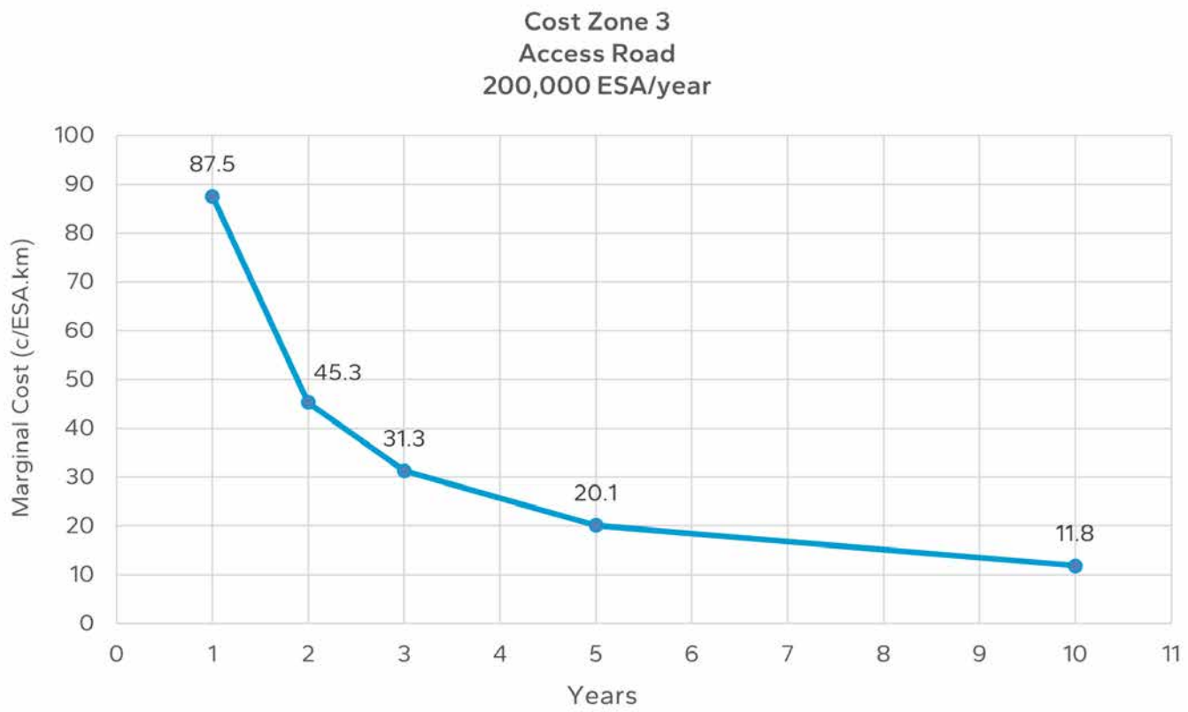
Figure B 9.4: Marginal cost chart for cost zone 3 access roads with 200,000 ESA/year loading
