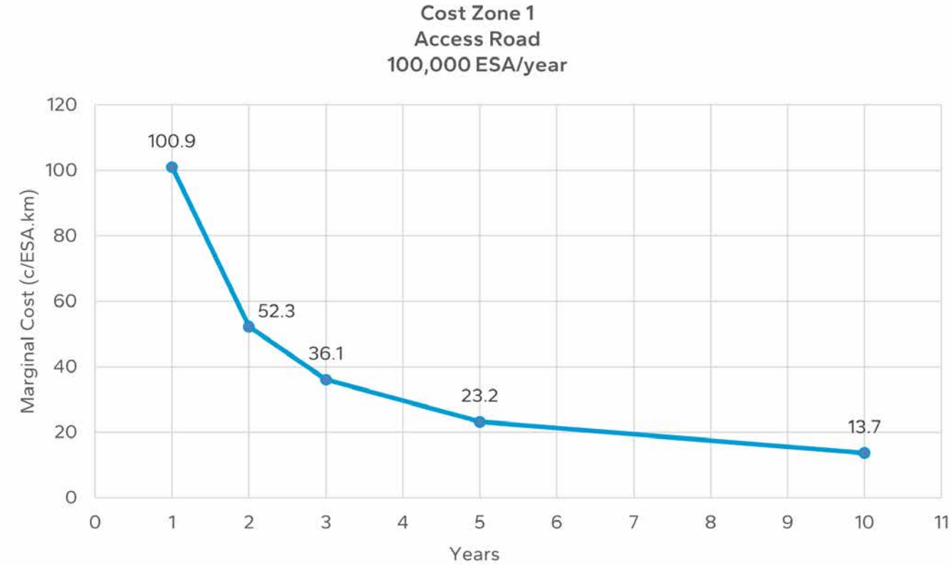
Figure B 1.3: Marginal cost chart for cost zone 1 access roads with 100,000 ESA/year loading
