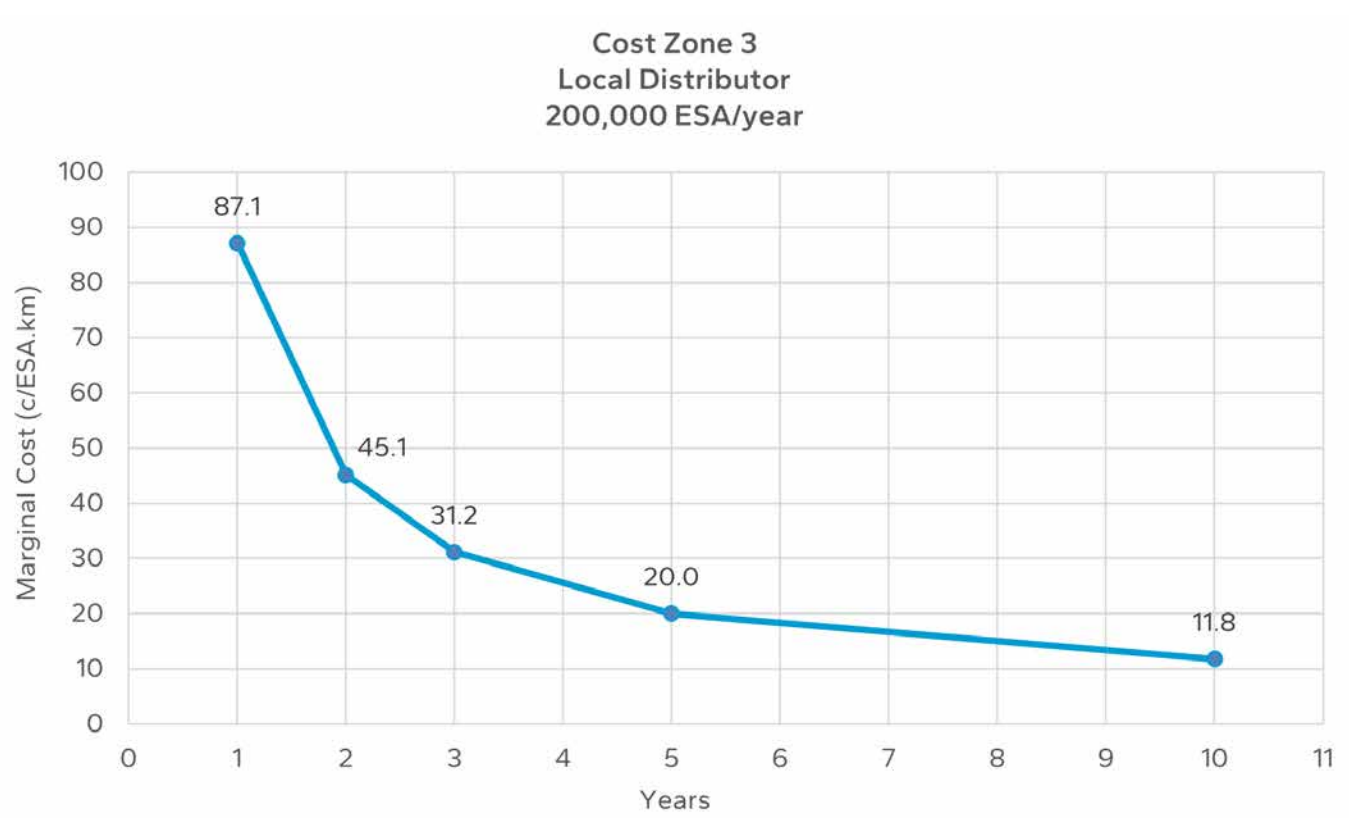
Figure B 10.4: Marginal cost chart for cost zone 3 local distributor roads with 200,000 ESA/year loading
