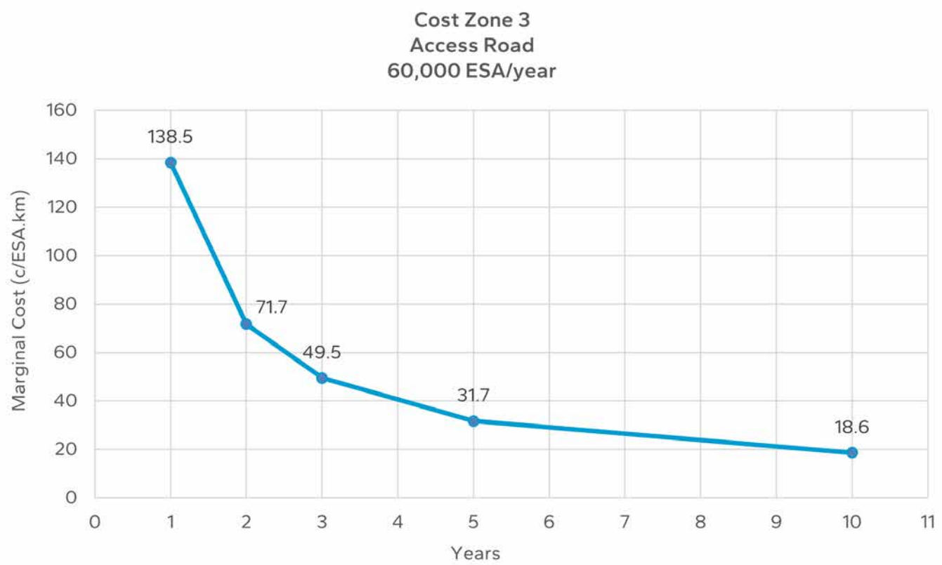
Figure B 9.2: Marginal cost chart for cost zone 3 access roads with 60,000 ESA/year loading
