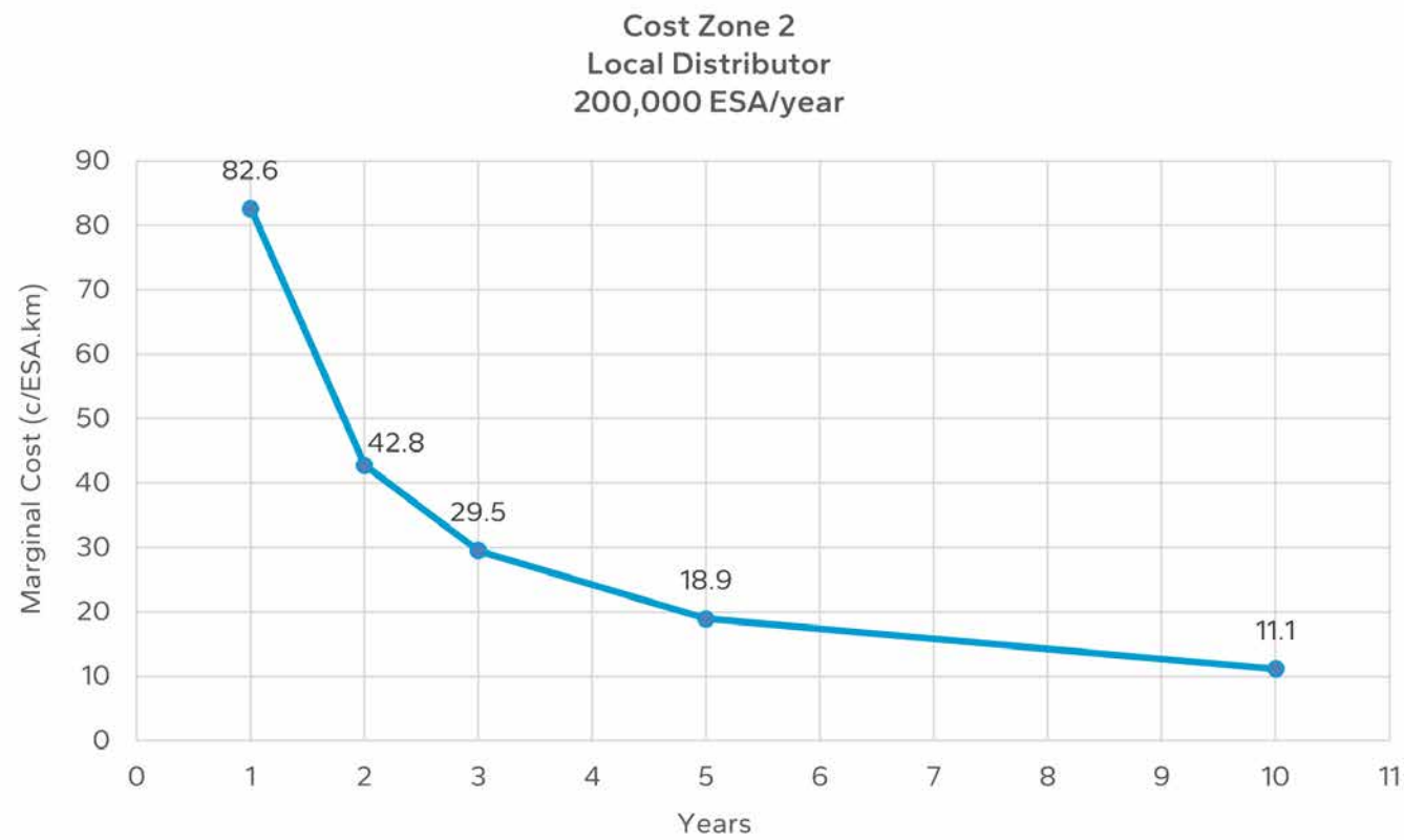
Figure B 6.4: Marginal cost chart for cost zone 2 local distributor roads with 200,000 ESA/year loading
