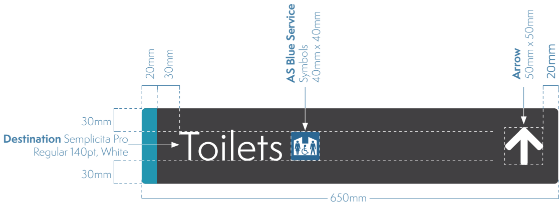
These signs panels can installed singularly or grouped. Panels can be shortened or lengthened to suit the application
