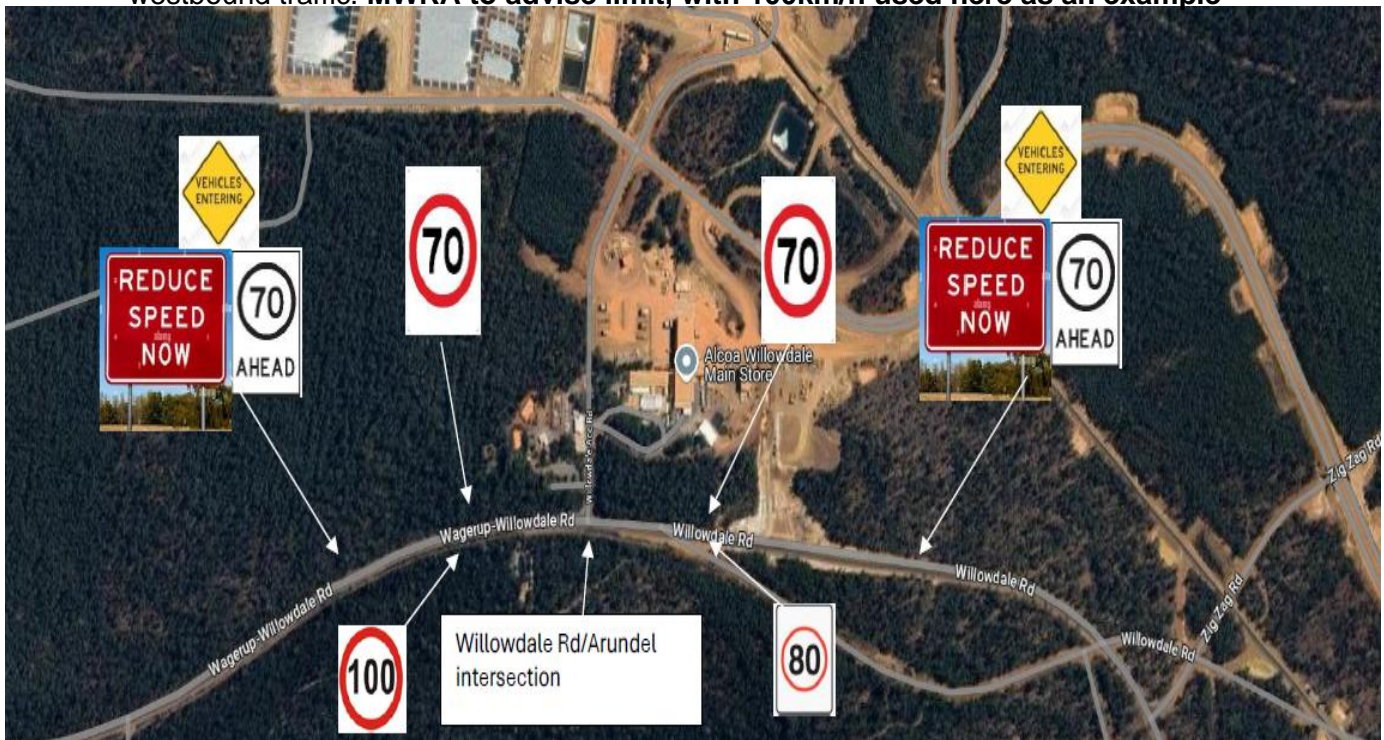
Fig. 1: Proposed installation of new speed limit signage for Willowdale road. East of the refinery access road turnoff for eastbound traffic, and west of the Arundel intersection for westbound traffic. MWRA to advise limit, with 100km/h used here as an example
