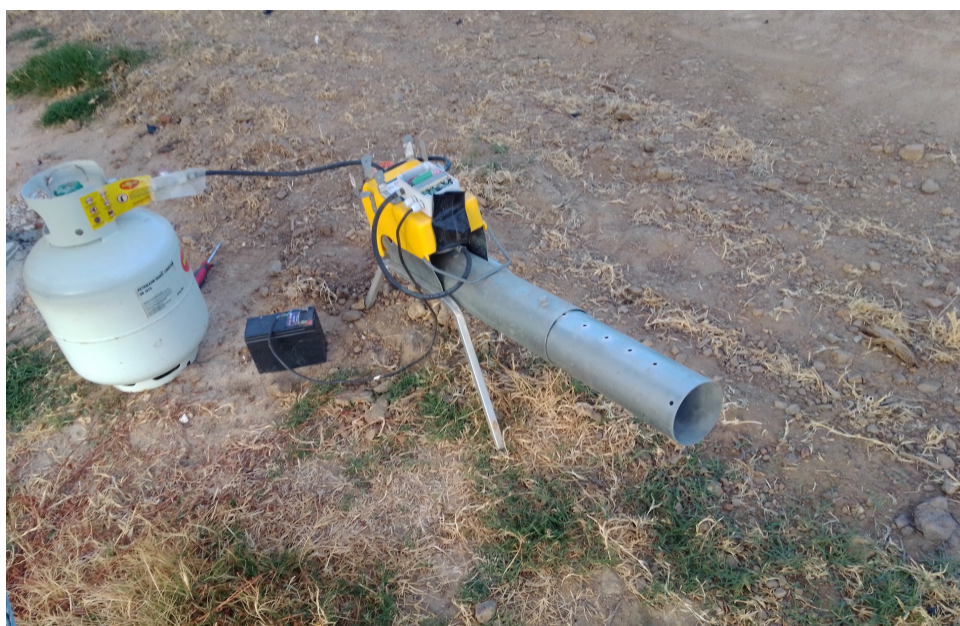
Figure 1: Zon Mark 4 gas cannon (tube length setting that was used for noise measurements)
