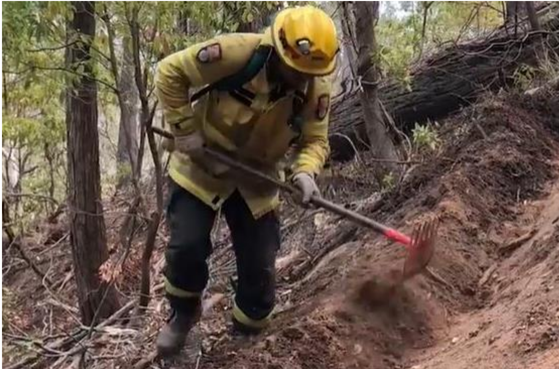
Figure 9: Example of rack hoe usage, note awkward posture and repetitive movements.
