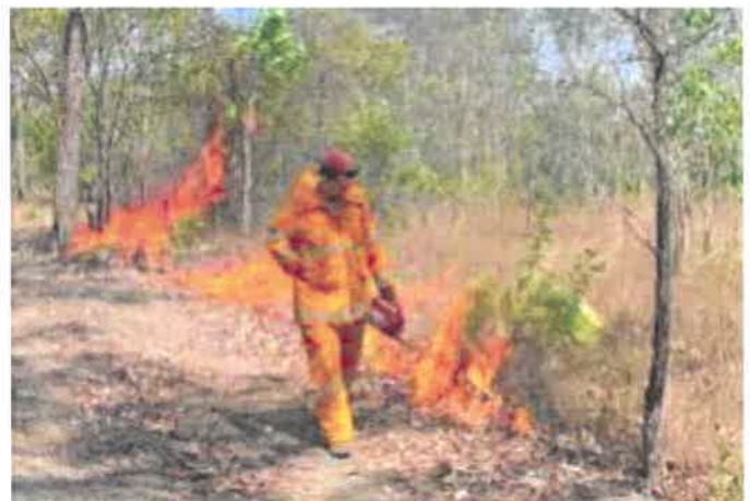
Figure 4: Example of drip torch operations.
